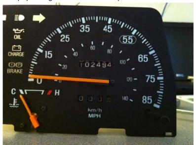
13. With the odometer correctly in position, re-heat up your knife and work the plastic back down over top of the odometer bar to hold it in place.
