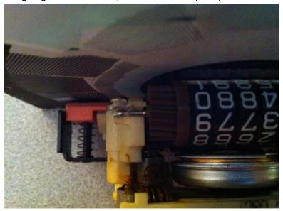
7. The odometer bar will now pop up on the left side, and pull out from the right side.
